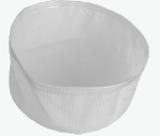
✓ Water-oil proof polyester cartridge filter, with external PTFE membrane providing 2.7 m2 surface and efficiency class H13.
